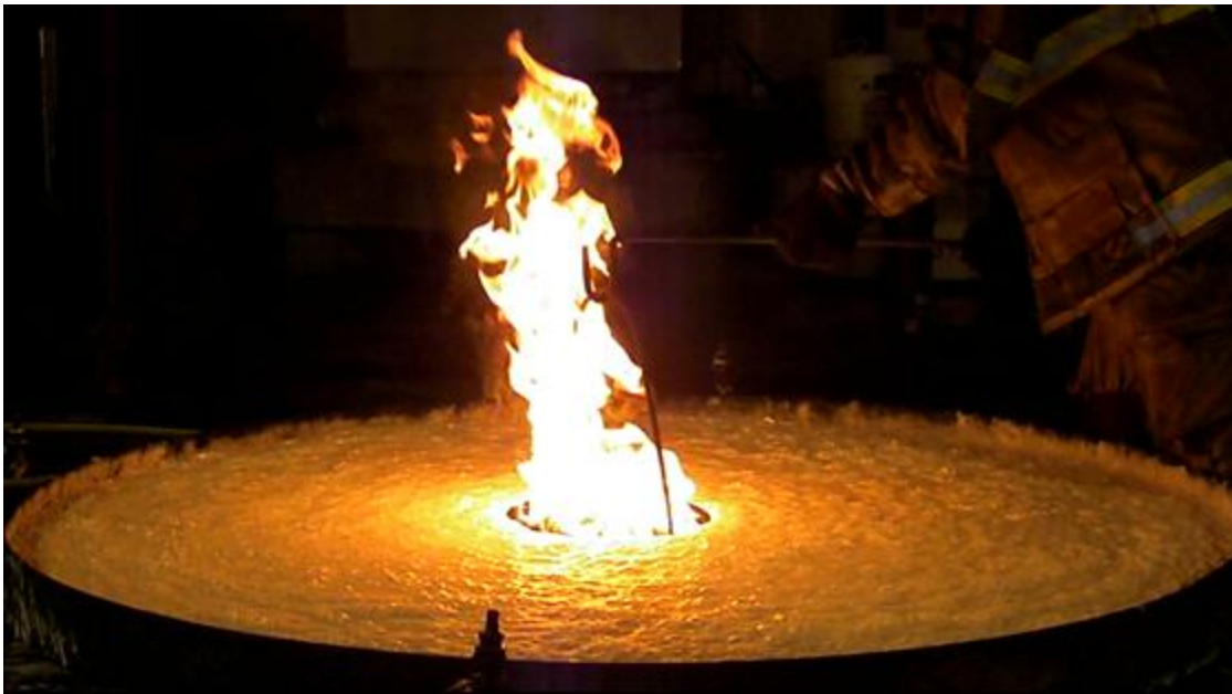
Figure 1: Firefighter placing the started pan in the foam-covered fuel at the beginning of the burnback test
